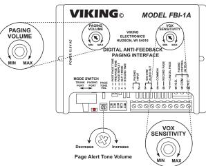
not accessed, the VOX sensitivity is set too high and should be decreased until the LED turns off (see **Programming** section **B**). During playback in either mode, the LED will light steady for the entire duration of the message playback.
