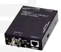
The E-TBT-FRL-05(xxHT) converter family contains simple "Plug and Play" converters used at the edge of a hardened network to provide 10Base-T Ethernet connections for legacy devices in challenging locations. Depending on the model, these converters can provide Multi-Mode or Single Mode fiber connections with SC or ST connectors for extended distance communications up to 40 kilometers. These converters ensure safe reliable operation in temperatures between -25°C and +70°C.
