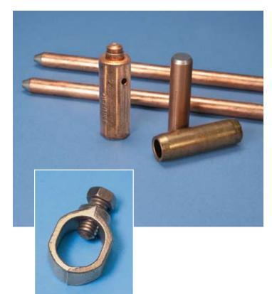
ERITECH® brand of copper-bonded steel ground rods resist corrosion and provide for a service life of more than 40 years in most soils. They are manufactured using ERICO's unique copper-bonding process which produces a reliable, long-lasting and extremely durable rod. ERITECH rods exceed the requirements of ANSI®/UL® 467-2004. CSA® and ANSI/NEMA® GR-1.
