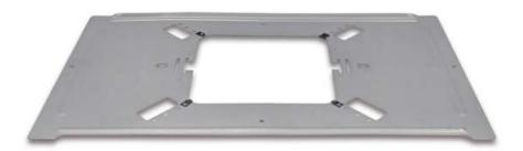
The SA-TBA is a tile bridge designed to mount 8 inch loud speaker and bridges both 2 ft x 2 ft and 2 ft x 4 ft ceiling tiles. It is compatible with the Viking models SA-1S, 30AE, 35AE, and 40AE speakers. The SA-TBA tile bridge is constructed of 24 gauge cold rolled steel with an electro galvanized rust-resistant finish.
