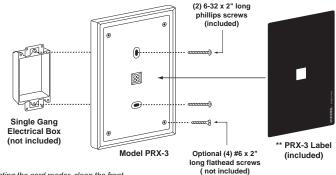
\*\* Important: After mounting and testing the card reader, clean the front recessed area of the unit with rubbing alcohol and apply the provided label. Please note, the label is permanent and not easily removed.
