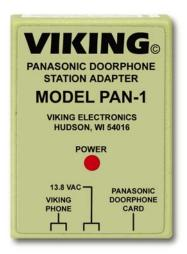
The Viking PAN-1 will allow a Viking "E" series speaker phone (E-10A, E-20B, E-30, E-35, E-40, E-50, E-60, E-65, E-70, E-75, etc.) to interface with Panasonic Doorphone/Door Station Cards.
