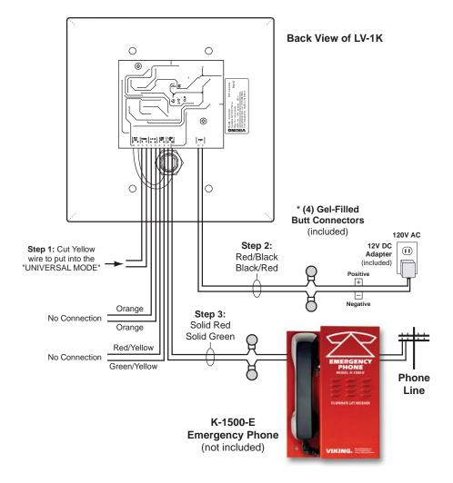
\* **Note:** The gel-filled (water-tight) butt connectors are designed for insulation displacement on 19-26 gauge wire with a maximum insulation of 0.082 inches. Do not strip wires prior to terminating.
