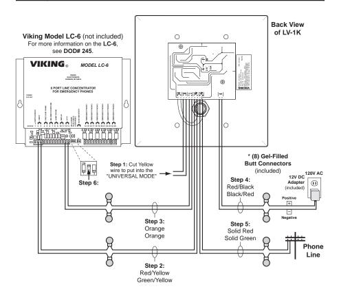
\* **Note:** The gel-filled (water-tight) butt connectors are designed for insulation displacement on 19-26 gauge wire with a maximum insulation of 0.082 inches. Do not strip wires prior to terminating.
