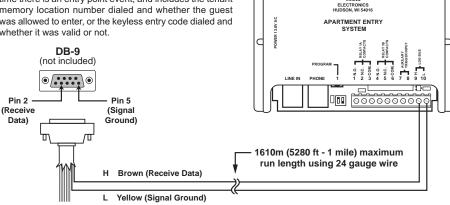
If the RS-232 input of a PC, printer, etc. is capable of receiving TTL level RS-232 signals, then the LOG BUS can be wired directly into the RS-232 "Receive Data" and "Signal Ground" pins to receive ASCII data. Windows "Hyper-Terminal" can be used to receive the data on a PC (use the settings in the chart) or visit www.vikingelectronics.com to download free ENTRY LOGGER software (see Operation section E, "Entry Logger Software").
