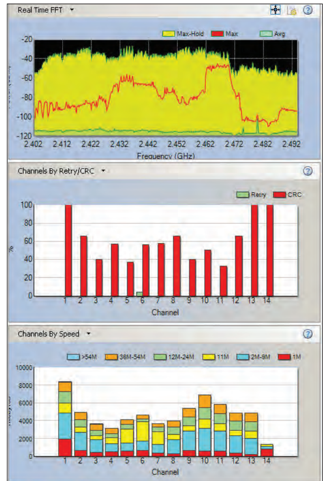
Figure 2: RF interference and Wi-Fi impact analysis
