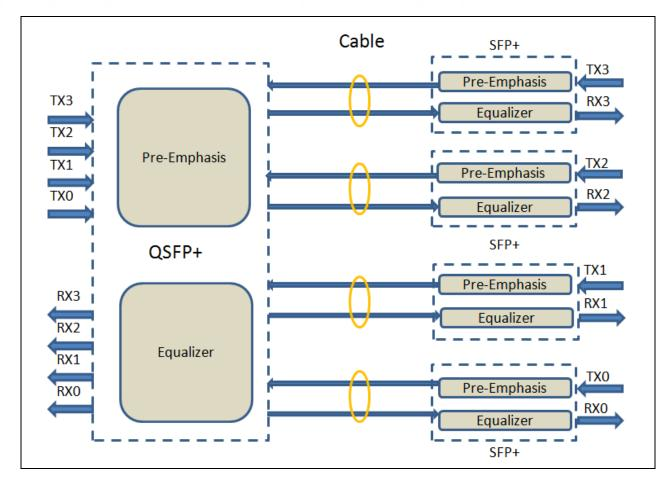
The transmitter side accepts electrical input signals. All input data signals are differential LVPECL or CML logic and they are internally terminated. The parallel input electrical signal first is processed via the Pre-Emphasis.
