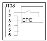
2. **+24 V Normally Open**: EPO is activated when an isolated SELV 24 VDC voltage is supplied on pin 1 with reference to pin 2. Connections: 3-5 and 4-6.
