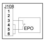
4. **+24 V Normally Closed**: EPO is activated when a SELV 24 VDC voltage is removed from pin 3 with reference to pin 4.
