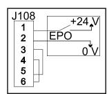
3. **Dry Contacts Normally Closed**: EPO is activated when a connection from pin 3 to 5 is opened. Connections: 4-6.
