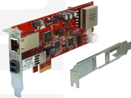
The N-GXE-POE-xx-01 Network Interface Card (NIC) provides connectivity to a secure fiber network while also delivering power to a PoE Powered Device (PD), such as a VoIP phone with a copper UTP interface. It fully complies with all IEEE 802.3z and 1000Base-X standards, providing up to 2000 Mbps full-duplex bandwidth capacity.
