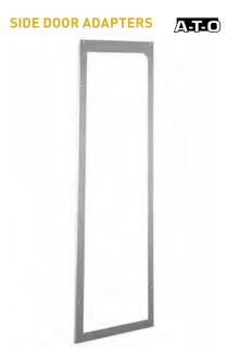
Side Door Adapters are made from 14 gauge steel and finished in RAL 7035 textured light-gray polyester powder paint. They allow the mounting of a standard door to the side of the enclosure. When mounted to the enclosure, they maintain enclosure environmental integrity.
