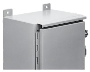
Protects door hardware from dripping water and settling dust. Attaches quickly and easily to the enclosure with stainless steel screws and sealing washers (hardware is furnished). Stainless steel hinge pin and stainless steel door clamping assemblies are furnished to replace the standard hinge pin and door clamping assemblies. A tube of sealing compound is also supplied with each kit. Manufactured from 14 gauge steel with an ANSI 61 gray polyester powder paint finish over pretreated surfaces.
