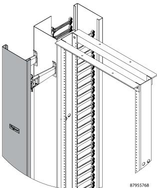
Rear cover is an accessory for all CABLETEK™ Vertical Cable Managers with post and gates. For double-sided managers, covers attach to included post and gates. For single-sided managers, appropriate Post and Gates Kit must be ordered.
