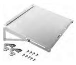
The shelf mounts to door using the Door Bar Grid Straps (sold separately). Shelf is 16 gauge steel with 12 gauge brackets. Shelf finish is RAL 7035 textured light-gray polyester powder paint. Locks in two positions—90 degrees as a shelf and 15 degrees as a writing surface. Also mounts to three-row grid straps, side or back panel, or any flat surface. Holds up to 30 pounds.
