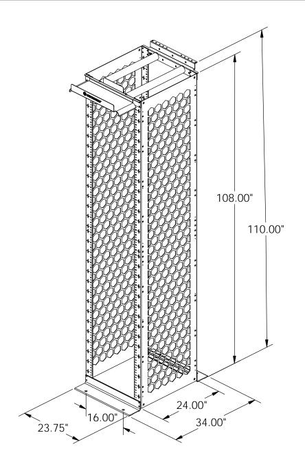
TESTED TO UL2416 WITH A WEIGHT LOAD OF 2000LBS.
