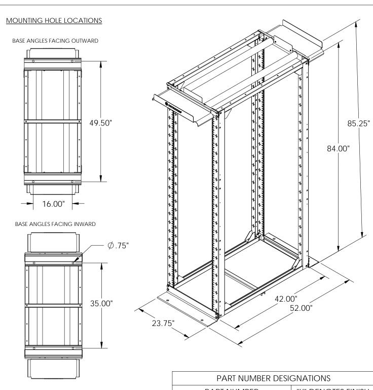
**TESTED TO UL2416 WITH A** WEIGHT LOAD OF 2000LBS
