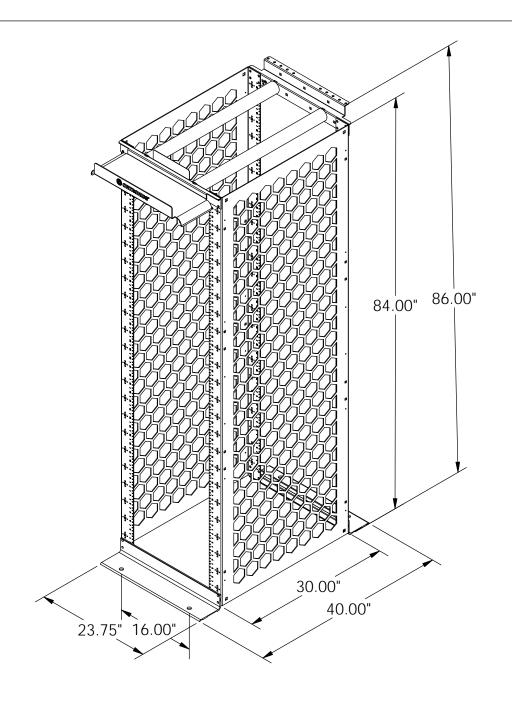
TESTED TO UL2416 WITH A WEIGHT LOAD OF 2000LBS.
