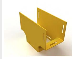
Vertical Tees are used to drop cables vertically from horizontal routes into frames or cabinets. They are available with and without covers. Vertical tees in 8" X 4" and 12" X 4" can be used to transition to smaller duct and retrofit tees can be installed where cables are already in place.
