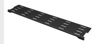
Zero rack unit horizontal managers slide into the slots in the Mighty Mo 20 fingers and provide support for fiber and copper cables exiting horizontal equipment modules. They toollessly lock into place with the 19" version mounting between 2 vertical managers in front of the equipment. Internal versions are sized to fit inside the vertical managers and provide a continuous horizontal path across the front of the racks and managers.
