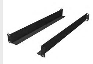
The 6" equipment support brackets can be cantilever mounted at the rear of any Mighty Mo rack and used to support equipment mounted to the front rails. Deeper equipment support brackets are sized to the 16-1/4" to 30" channel racks and 4-point mount with the equipment's mounting ears to provide zero unit support from front to back.
