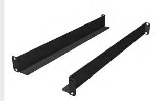
The 6" equipment support brackets can be cantilever mounted at the rear of any Mighty Mo rack and used to support equipment mounted to the front rails. Deeper equipment support brackets are sized to the 16-1/4" to 30" channel racks and 4-point mount with the equipment's mounting ears to provide zero unit support from front to back.
