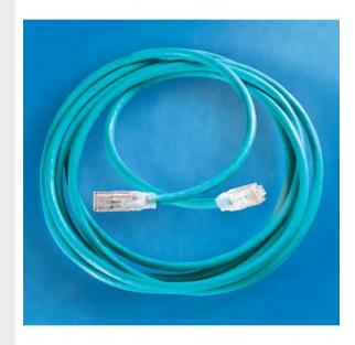
Clarity 6 Modular Patch Cord, blue, 5', Category 6, four-pair UTP stranded 24 AWG PVC/CM, center tuned with Clarity 6 connecting hardware for optimum Category 6 installed performance using Ortronics Paralign 2 pair-positioning technolgy
