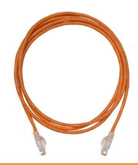
Clarity 6 Modular Patch Cord, orange, 5', Category 6, four-pair UTP stranded 24 AWG PVC/CM, center tuned with Clarity 6 connecting hardware for optimum Category 6 installed performance using Ortronics Paralign 2 pair-positioning technology
