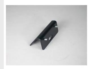
Cable retention bracket providing lances and hook/loop fasteners is designed for use when installing backbone cables from below fiber cabinet. Mounts to bottom rear of fiber cabinet to provide robust fastening point for incoming backbone cables. Suitable for use with 2U, 3U and 4U rack mount fiber cabinets.
