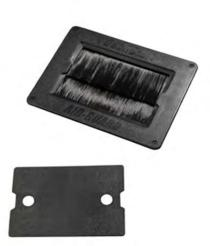
Air Guard Brush Cable Grommet, flush mount Extreme is a heavy duty unit with a two stage, integrated sealing system, EPDM gasket material (UL94HF-1 rated) and standard Air Guard brush technology, to provide the most effective air seal.
