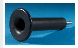
This spool has a #12-24 stud, black, molded in place and can be threaded into the EIA holes on any Ortronics rack. Use it to mount cable management panels, patch panels or screw it in anywhere additional cable management is desired.
