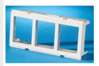
This plate accepts three TracJack modules or blanks. Use with OR-40700071, OR-40700072, or OR-40700073 bezels, to snap mount into 2.70" x 1.375" TIA referenced furniture openings for Steelcase, Haworth, Knoll and others.
