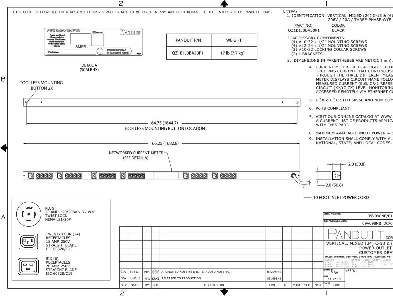
1. IDENTIFICATION: VERTICAL, MIXED (24) C-13 & (6) C-19 NETWORKED 208V / 20A / THREE-PHASE WYE POU
