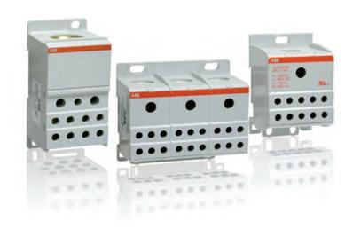
Using a Distribution Block eliminates the need to wire each device in the control circuit back to the power source by using one large wire on the input side, and several smaller wires on the output side to your devices downstream. This will give your electrical panel a clean and professional look.
