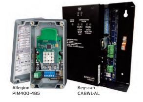
virtually anywhere. It is easily connected to your LAN/WAN network and can be powered using PoE (where available). If PoE is not available a 12VDC input option is provided.
