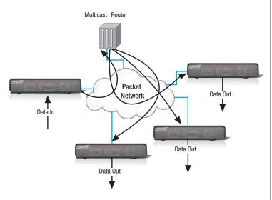
**3.2** The Multicast capability also means that the PacketBand can separate the clock recovery data from the bulk user data. This means larger networks with multiple "hops" can deliver not only improved clock Synchronization, but there are network design/loading/QoS and resiliency benefits as well.
