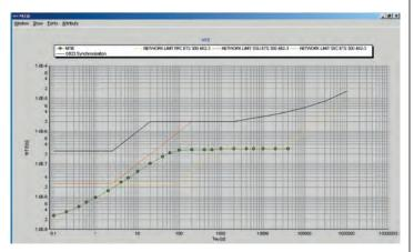
Actual MTIE report from a customer's testing showing excellent adaptive clock results with PacketBand being close to the PRC reference source and significantly lower than the G.823 Synch mask.
