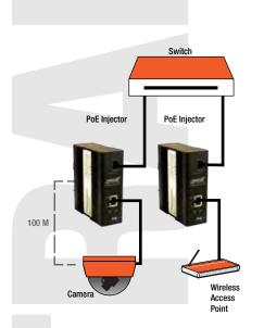
SI-IES-111D-LRT has one SFP slot and one RJ45 port. The RJ45 port supports 802.3at (PoE+), and can provide 30W for high powered application. The SFP slot provides more flexibility when planning and implementing the network. The slot can accept either a 100m or 1000m SFP module. This makes it possible to easily change the transmission mode and distance of the connection by using a different module. The SFP module is hot-swappable, and there is a dip switch to adjust the LFP function.
