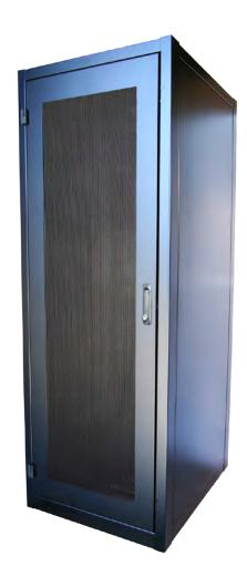
R. F. Mote Series Seismic Zone 4 Kitted Cabinets (30" and 24" Wide) are independently certified to meet UBC code seismic strength requirements for Zone 4 as per Bellcore GR-63-CORE specifications. Standard kitted Seismic cabinets include: 2 Perforated doors, 2 solid side panels, 2 pair cage-nut style mounting rails, levelling feet, cover plates, and hardware package.
