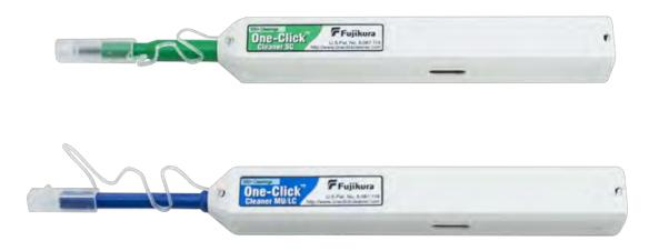
The Fujikura One-Click<sup>™</sup> cleaners are mechanical cleaning tools designed to clean connectors residing in an adaptor or faceplate and unmated connectors. The Fujikura One-Click<sup>™</sup> cleaners use a novel dry cleaning strand to gently sweep and lift away dust and residues from the connector end face.
