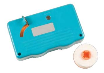
The Cleanreel cassette cleaner is the perfect solution for cleaning fibre connector endfaces and will clean all standard 2.5mm and 1.25mm connector types. A simple squeeze of the lever opens a window to reveal a fresh section of anti-static micro-fibre cloth. The connector end-face is then stroked along the cloth in one direction to give a perfect clean. Each cassette cleaner contains a replaceable reel of cloth with each reel giving up to 400 cleans before it needs replacing.
