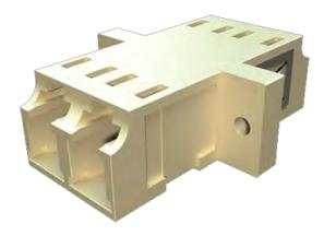
Our range of LC adaptors have high precision alignment sleeves for improved reliability and better reconnectability. The LC adaptors come with ceramic sleeves for both singlemode and multimode. The housing is available in different colours with options for flange or flangeless body and metal or inbuilt clips.
