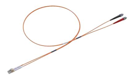
Multimode patch cords are used to connect high speed and legacy networks like gigabit ethernet, fast ethernet and ethernet. Multimode patch cords are manufactured using LSZH cable and conform to IEC, EIA TIA or Telcordia standards. OM2 patch cords are terminated with standard connectors giving optimum optical performance.
