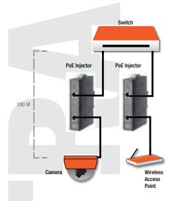
The SI-IES-1200-LRT is a industrial grade 1-port 10/100/1000Base-T PoE+ Mid-span Injector which provides a simple solution to enabling the existing infrastructure with IEEE802.3at PoE+ capability. Transition Networks' Industrial Mid-span Injectors are designed to reliably operate in harsh environments such as those found on factory floors, out-door enclosures or other hazardous environments.
