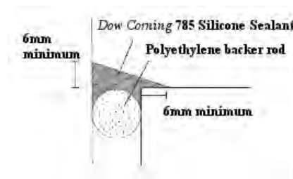
Figure 1: Fillet Joint.
