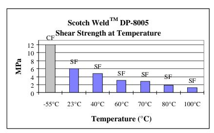
The above overlap shear tests data was collected on 5mm\*100mm\*25mm PP specimens overlapped 12.5mm, allowed to cure at 24°C for 7 days and then tested at a rate of 10mm/mn in overlap shear mode, at the temperature shown.
