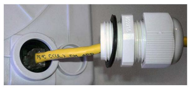
Once the RJ45 connection has been made, screw in the gland into the housing making sure it is tight enough for a water tight seal but not so tight to cause the rubber seal to squeeze off.
