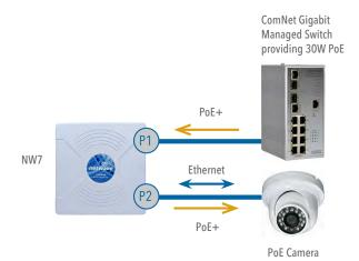
Note: The Power Injection Module (PIM) provided only supports speeds up to 100 Mbps. To utilize the full speed of the Gigabit Ethernet ports, you will need to connect the radio to a Gigabit POE switch.
