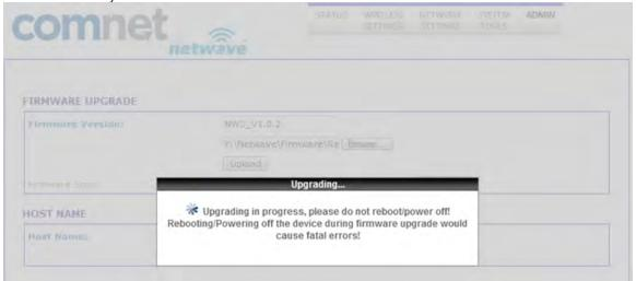
NOTE: If a firmware upgrade is being performed on a node connected on the remote end of a wireless connection, it may take several minutes for this screen to clear as the link needs to re-establish and connections to restart. One may have to clear ARP cash on the connected PC by issuing arp -d command at the command prompt.
