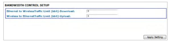
Enter in the throughput limiting values for upload and download then hit the Apply Setting button. This feature could be useful when configuring clients connecting to a single multipoint AP or in a repeating system thus keeping within the maximum throughput of any one hop or multipoint AP.
