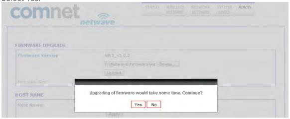
» The following screen will now show reminding the user to not reboot during an upgrade process. This screen should render for at least 60 seconds if the PC browsing to this particular node is locally connected.
