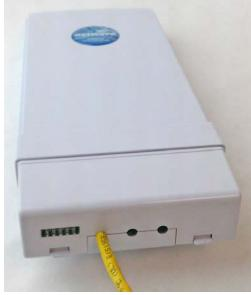
Connect one end of an RJ-45 Ethernet cable to the LAN OUT port of the Power Injection Module (PIM) and the other end to LAN of the access point - as sown below.
