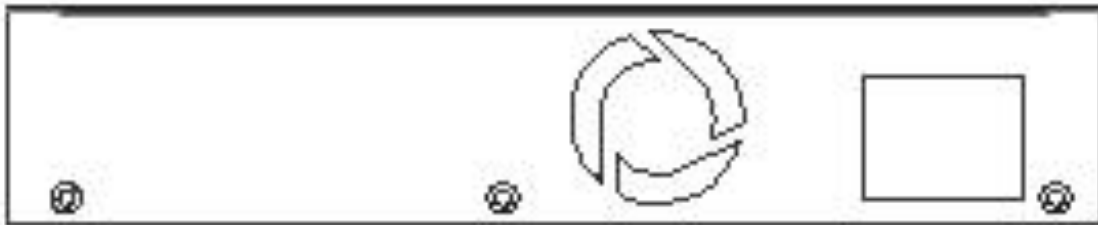
Rear panel of the CWGE9MS managed Ethernet switch
