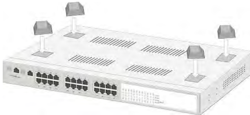
Attaching Rubber Feet to each corner on the bottom of the Switch
