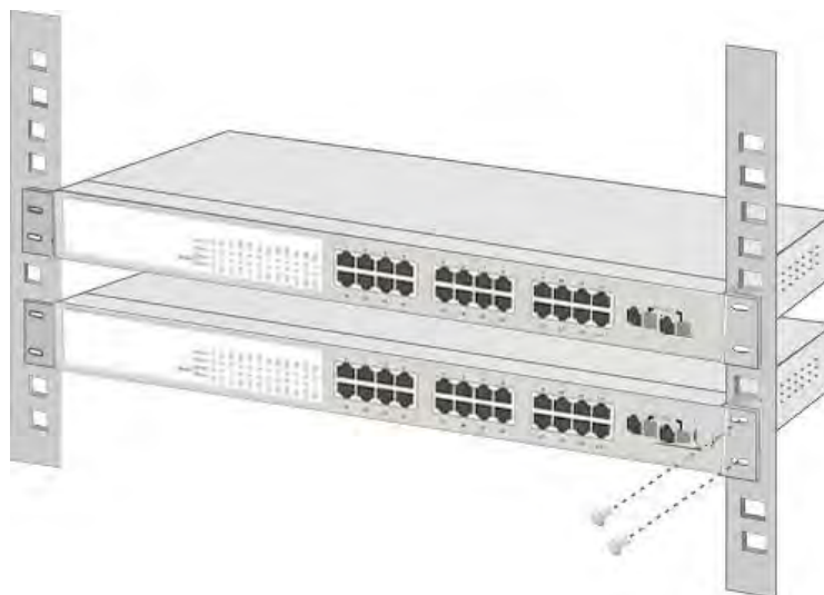
Mount the Switch in 19" Rack
