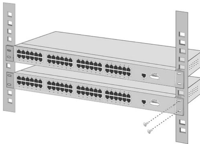
Mount the Switch in an EIA standard 19-inch Rack
