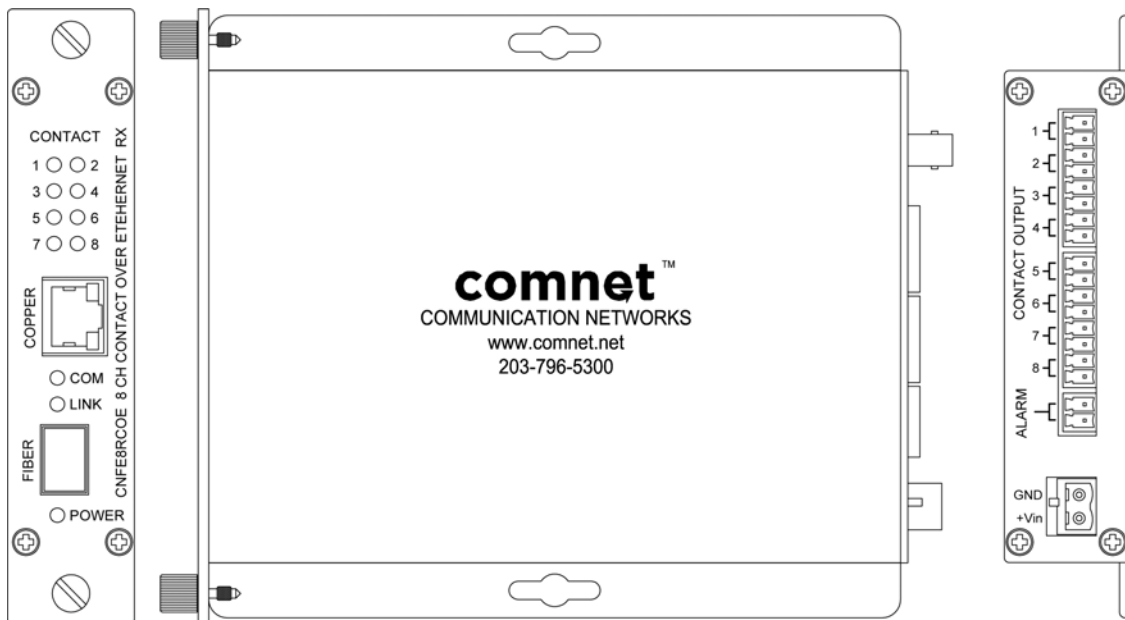
Mechanical Drawing of CNFE8RCOE MODULE
