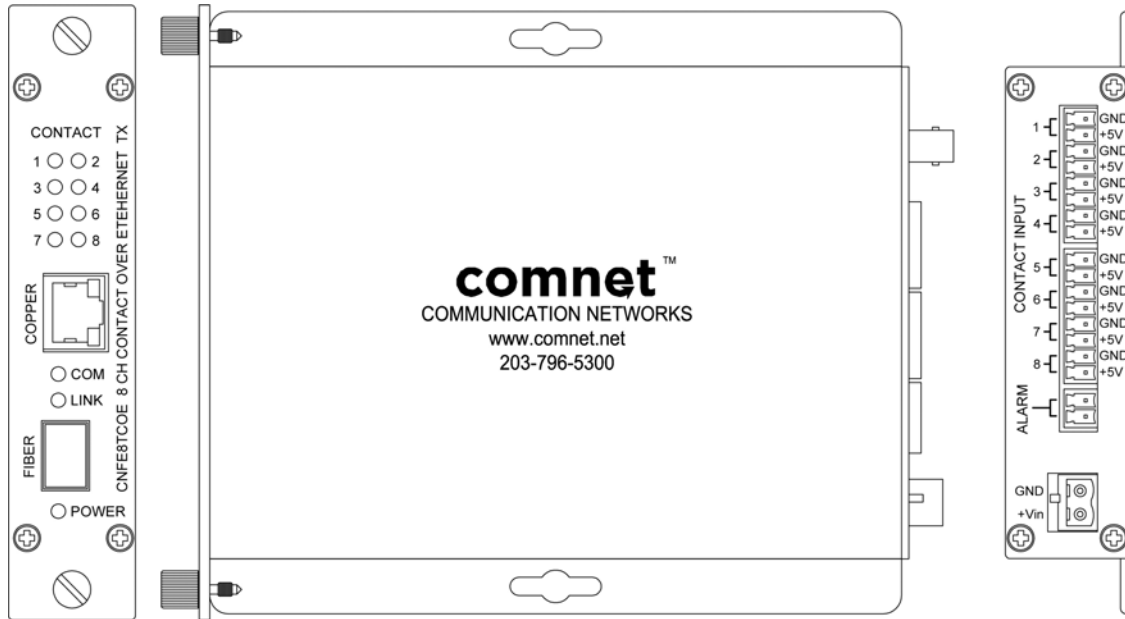
Mechanical Drawing of CNFE8TCOE MODULE
