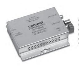
The ComNet<sup>™</sup> FVR10M video receiver detects an AM video signal on one multimode fiber optic cable. The receiver utilizes Manual Gain Control and is compatible with the ComNet FVT11M and the FVT20 transmitters. Plug-and-play design ensures ease of installation requiring no electrical or optical adjustments. Bi-color (Red/Green) LED indicators are provided for rapidly ascertaining equipment operating status. These units are only available in stand-alone configurations.
