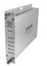
The ComNet<sup>™</sup> FVT/FVR40SFP series optical video link provides four 10-bit mediumhaul quality digital video channels, using optical SFPs for fiber type, connector, and distance. Plug-and-play design ensures ease of installation and no electrical or optical adjustments are ever required.
